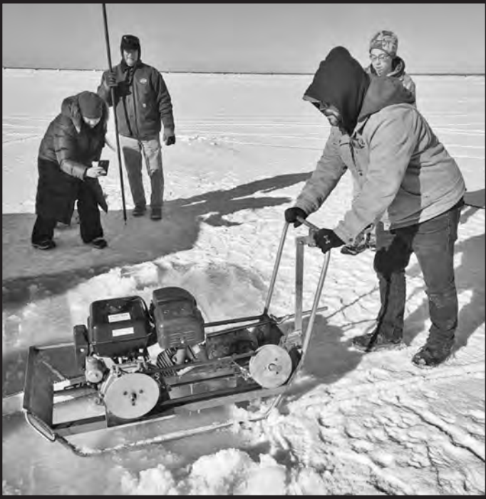
This sled saw is powered by a 13 hp motor and cuts with a 42 chainsaw bar.
